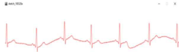
Figure 8. Live ECG signal using AD8232 heart beat sensor and Arduino
