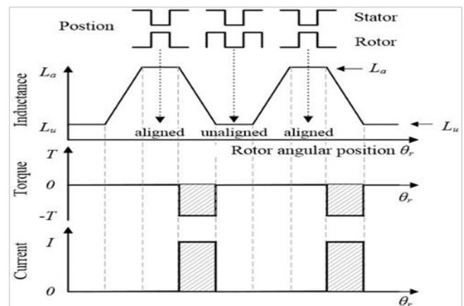
**Fig. 3: Torque relationship between the idealized inductance profile and the phase current. [21]**
