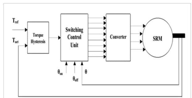
Fig. 5: Simple Block diagram of DITC [58]
