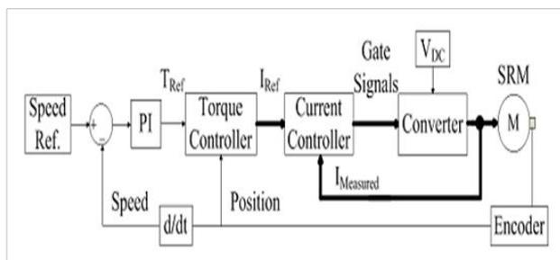
Fig.4: Indirect Torque Control for SRM [44].
