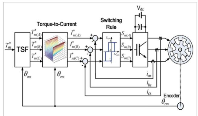
**Fig.6: Block diagram of torque minimization with TSF [27]**
