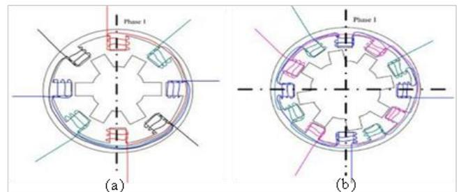
**Fig.2: Switched reluctance generator structure (a) four-phase 8/6, (b) three-phase 12/8 [3]**
