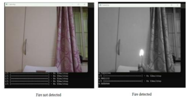
Fig. 7: Example of Fire Detection Using Deep Learning Methodology
