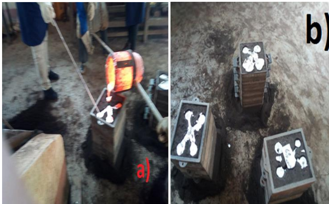
Figure 1: a) Pouring of the molten composites inside the mold b) Mould filled with molten composites c) Composites samples produced.
